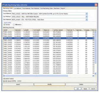
Machining parameter data is automatically drawn from the library as operations are created.
